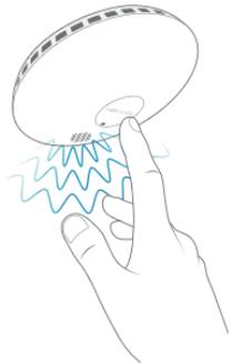
**EN** You should test the smoke detector every month to ensure that it is properly installed and working correctly. You can carry out the test directly on the detector by pressing the central button for three seconds. Note that the alarm will sound for eight seconds, protect your ears. If the alarm does not sound, check that the batteries are functional (see Troubleshooting on pages 12-13). Do not use a flame due to the risk of damaging the detector.
