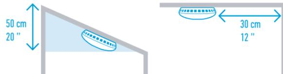
**EN** You are advised to fit the detector on the ceiling. Ensure that the chosen location is at least 30 cm from the wall. In case of a sloping ceiling, fit the detector no more than 50 cm below the highest point.
