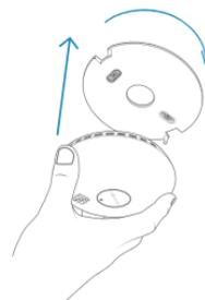
**EN** Then fix the detector to the plate by turning until it locks in place.
