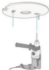
**EN** Position the mounting plate in the final location (instructions on pages 4-5) and mark the holes. Drill the holes and insert the plugs provided.
