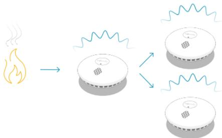
**EN** For maximum safety, you can connect your smoke detectors together. If smoke is detected, the alarm spreads to all the other smoke detectors in the house. **Note: a Somfy Protect security system is required to connect several smoke detectors together. The Somfy Protect app is used to connect smoke detectors.**
